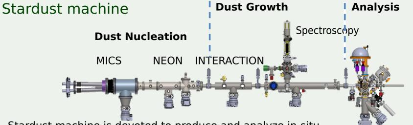
Stardust machine is devoted to produce and analyze in-situ highly-controlled analogs of the cosmic-dust in a versatile ultra-high-vacuum experiment. In this environment we will mimic the nucleation of the aggregates and the interaction they may experience with the circumstellar gases.
